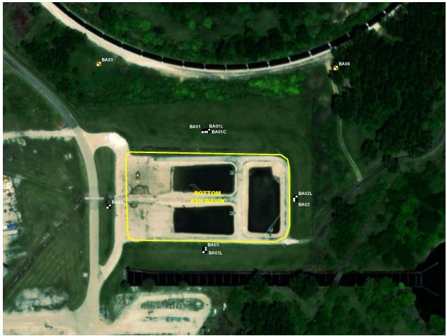
**Figure 2.1 Groundwater Monitoring Well Locations – BAB.** BAB = Bottom Ash Basin. Source: Ramboll US Corp. (2021a).
