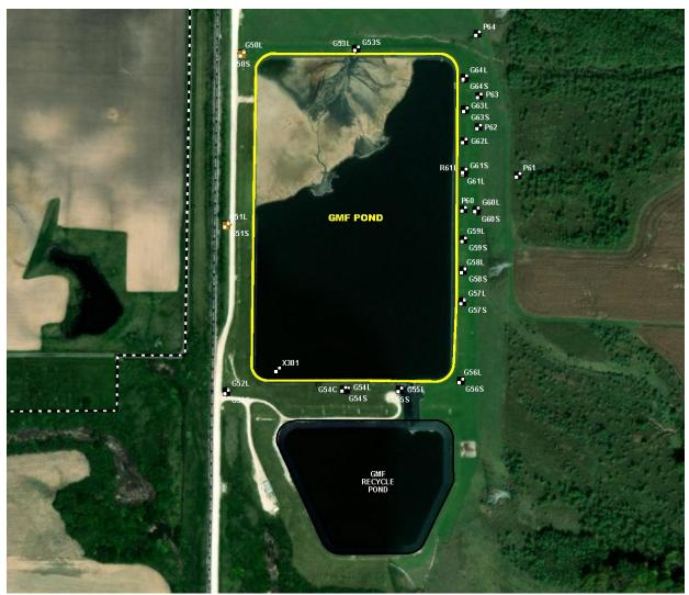
**Figure 2.2 Groundwater Monitoring Well Locations – GMF**. GMF = Gypsum Management Facility. Adapted from: Ramboll US Corp. (2021b).
