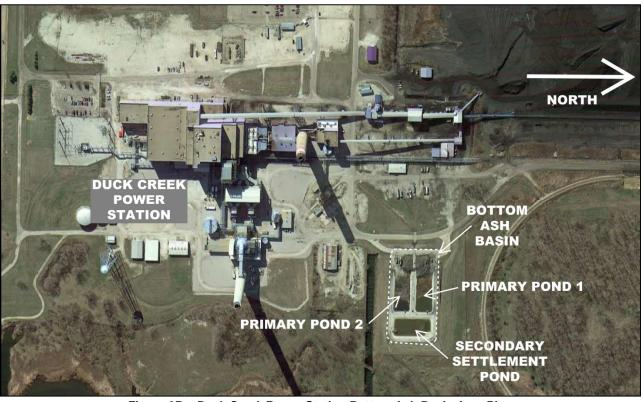
Figure 2B – Duck Creek Power Station Bottom Ash Basin Area Plan (Imagery from Google Earth Pro, 2016)
